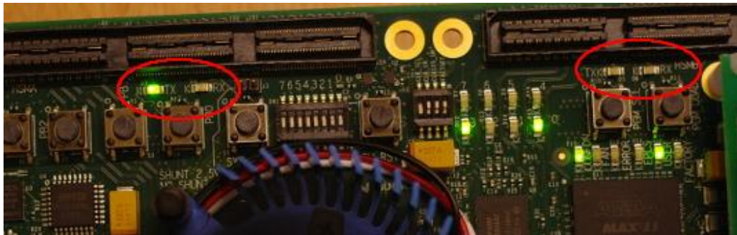
Figure 28. Red Circles Indicate the Four Link LEDs
