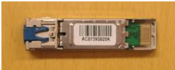
Figure 4. SFP Module for Single Mode Fiber Optic Cable (Blue Latch)
