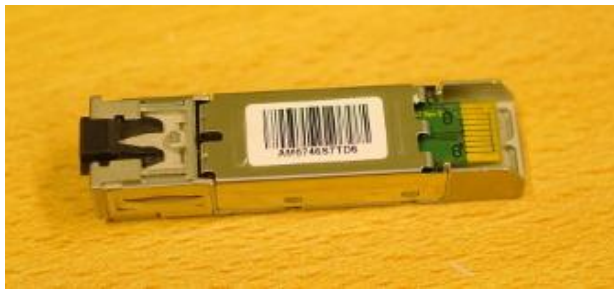
Figure 3. SFP Module for Multimode Fiber Optic Cable (Black Latch)
