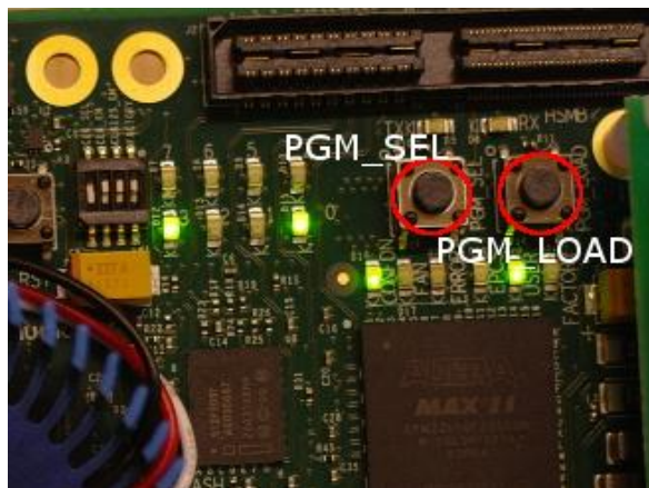
Figure 18. PGM_SEL and PGM_LOAD Buttons
