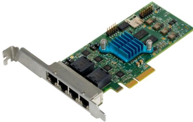
**Figure 6. FRS SoC Evaluation Board interfaces are named CE01, CE02, CE03, and CE04. Interface numbering starts from left.**
